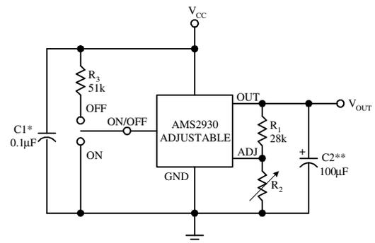
$$V_{OUT} = V_{REF} \times (R_1 + R_2) / R_1$$
