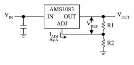
$$V_{OUT} = V_{REF} (1 + R2/R1) + I_{ADJ}R2$$
