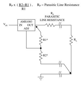
\*CONNECT R1 TO CASE CONNECT R2 TO LOAD
