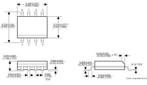
\*DIMENSION DOES NOT INCLUDE MOLD FLASH. MOLD FLASH SHALL NOT EXCEED  $0.006"\ (0.152 \text{mm})$  PER SIDE
