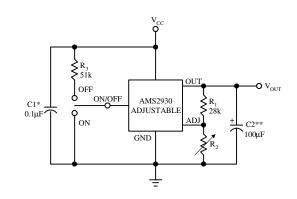
$V_{OUT} = V_{REF} \times (R_1 + R_2)/R_1$
